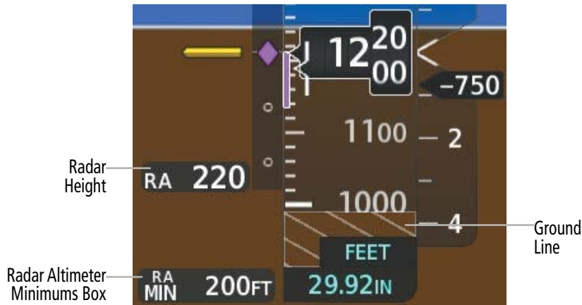
Figure 2-55 Altimeter Displaying Ground Line (Radar Altimeter Installed)
