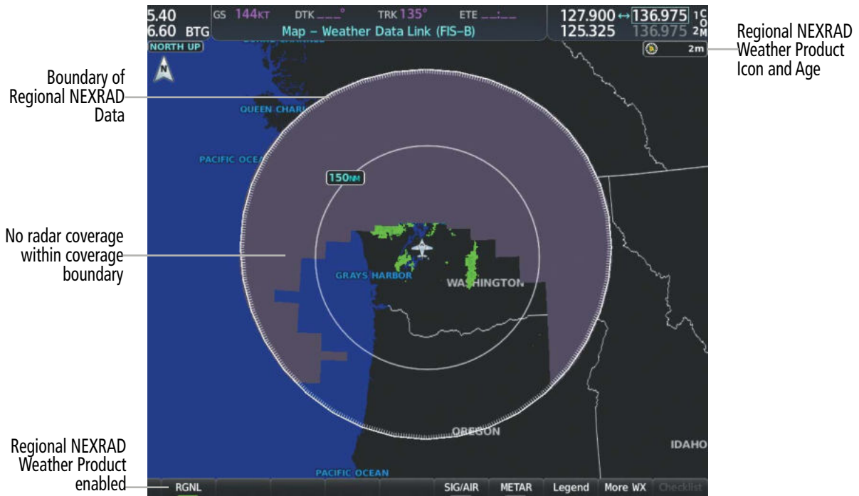
Figure 6-14 Regional NEXRAD Weather Product on the 'Map - Weather Data Link (FIS-B)' Page
