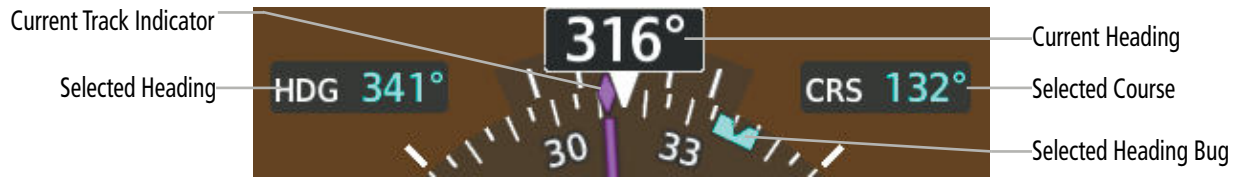
Figure 2-18 Heading and Course Indications
