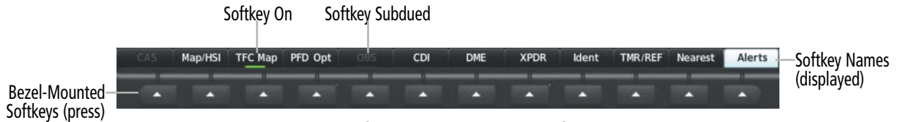
Figure 1-10 Softkeys (First-Level PFD Configuration)
