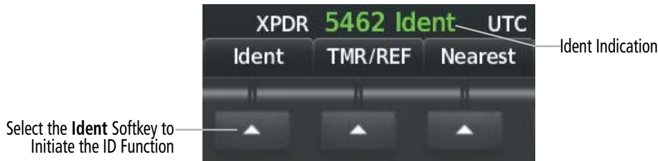
Figure 4-24 Ident Softkey and Indication
